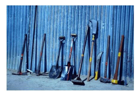
The poor labourers were struggling to achieve the standard excavation task rates with these worn out tools with poor handles. Construction quality hand tools with properly designed handles should be provided as shown above right to achieve productive output.
