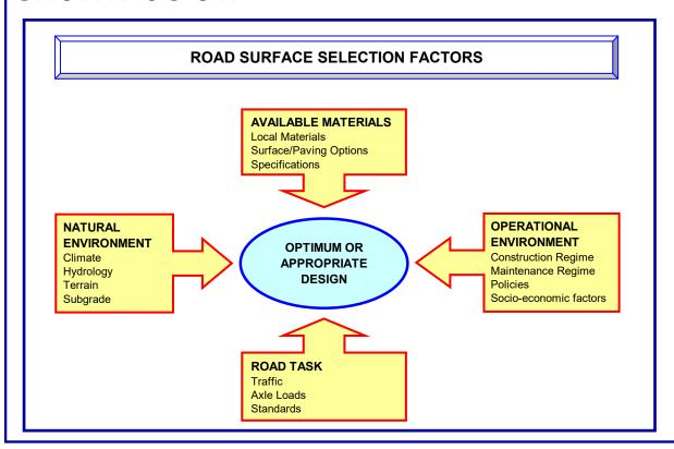
Local guidelines should be developed based on **Whole Life**Costing of the various feasible surface/paving options, including realistic maintenance assessment.
