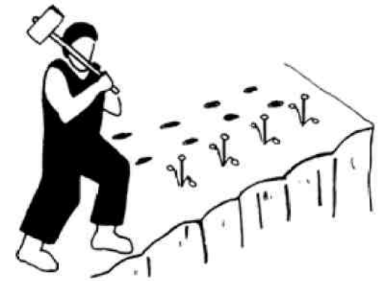
FEATHERS AND A PLUG IN GROUPS OF FOUR TO BREAK ROCK ALONG A LINE
